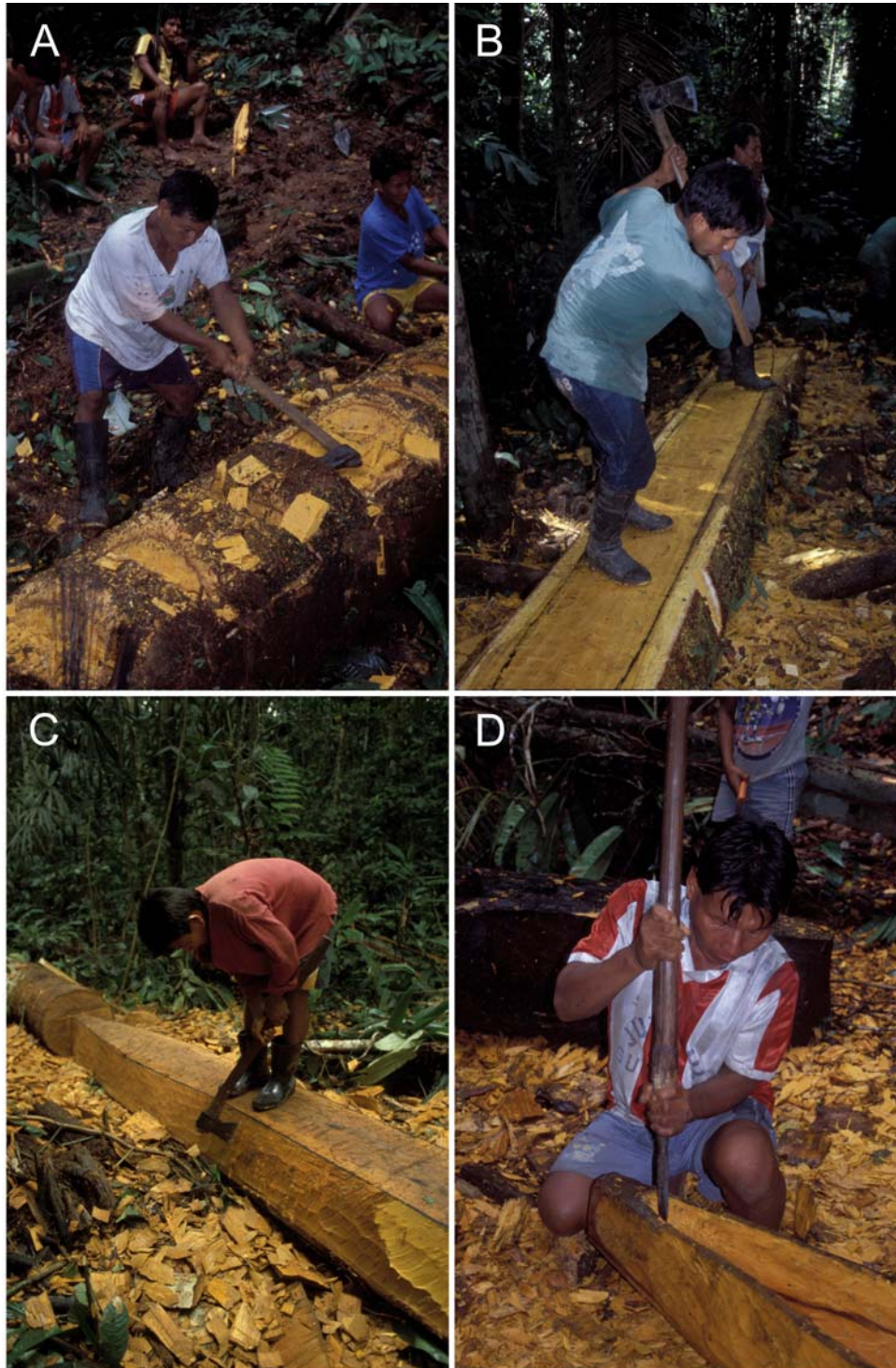
Figure 4-5. Steps in the construction of a dugout canoe ( you ). A. Initial cutting of the felled trunk. B. Removing wood from the sides of the felled trunk. Note the traced shape of the canoe (in black) on the top surface of the felled trunk. C. Continuing to remove wood from the sides of the felled trunk shaping the bow and stern into flattened points. D. Removing wood from the inside of the felled trunk creating a cavity ( you yacu ). Note the use of a you totecou , a chisel that is attached to a long pole or handle (All Photos by M. Gilmore).
