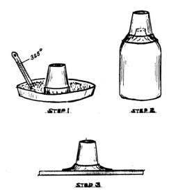
Step #1—Soften rim of pot in salt heated to 325 degrees. Step #2—Flare rim of pot over neck of a bottle. Sep #3—Complete flare by pressing pot flat on table.
